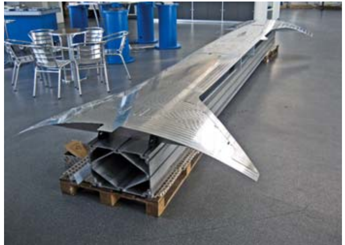
Aircraft bottom panel, machined in our subcontracting division mounted on ALUQUICK Large in preparation for measuring.
