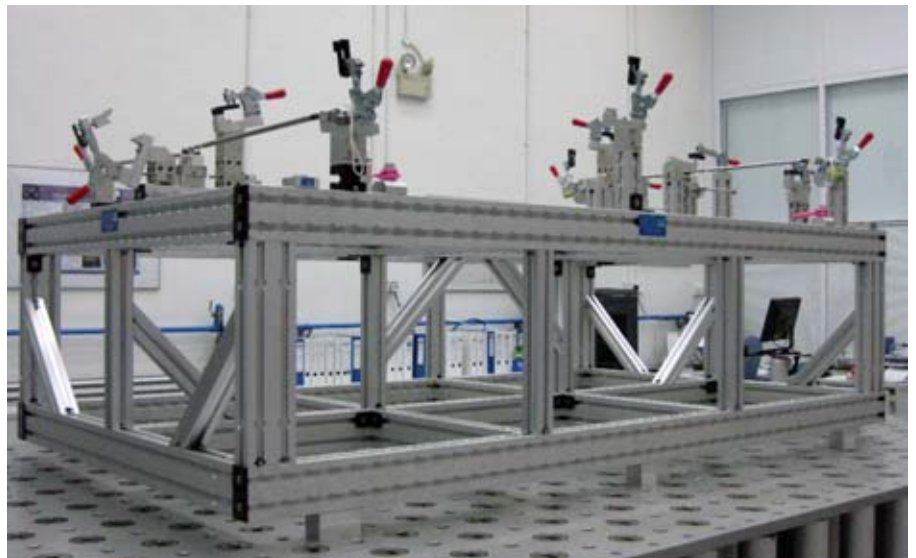
Frame type measuring fixture in ALUQUICK for roof mounted on a Witte sandwich plate
