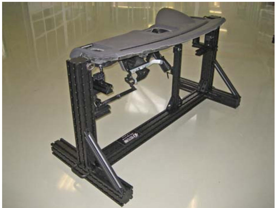
Instrument panel mounted on ALUQUICK 50x50 profiles with grid
