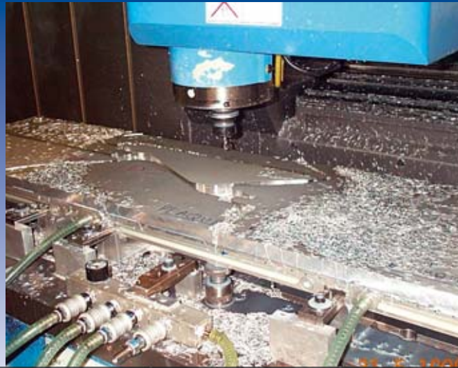
Vacuum grid type plate with additional threaded bores
