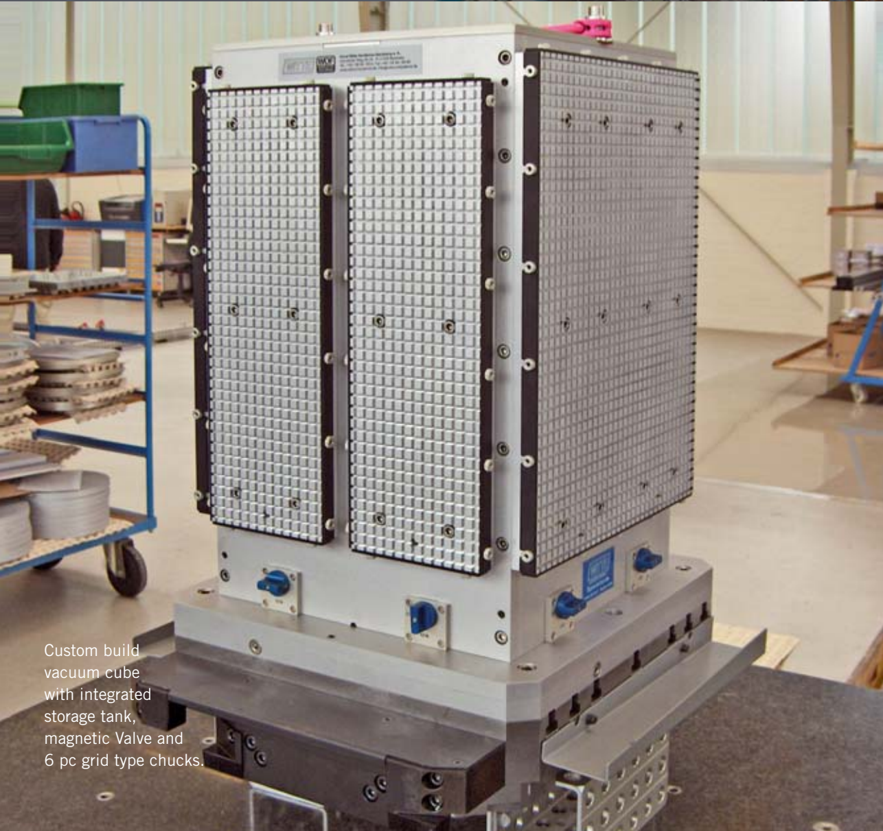
Vacuum grid type plate with additional threaded bores
