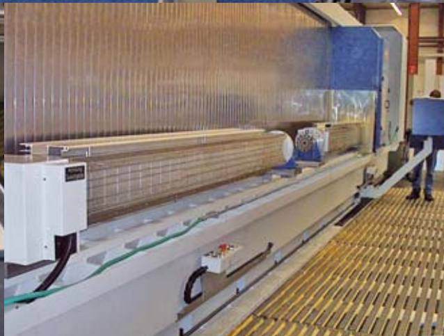
2 Rotating systems (each 3500mm) with vacuum clamping areas on all four sides for machining aluminium profiles
