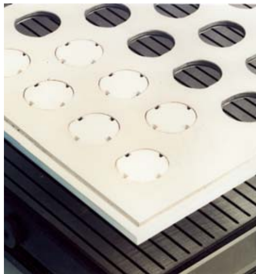
Slot vacuum chuck with special adapter plate
